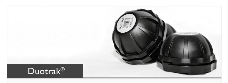
Duotrak® offers the possibility to measure in two positions, which can be essential in i.e. work places, where the radon concentration is required to be measured separately during working hours and non-working hours. Duotrak can be ideal for occupational radon dosimetry due to the possibility to have the detector in the ON-position only during working time.
